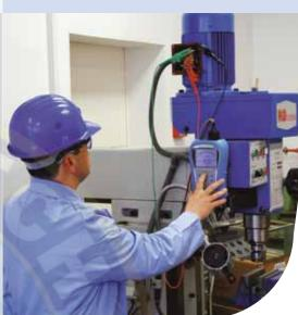
The MI 3121H Smartec 2,5 kV Insulation / Continuity is the portable measuring instrument for complete diagnostic testing of insulation and continuity measurements. Due to insulation resistance measurement with the test voltages up to 2.5 kV (measuring range is up to 100 G $\Omega$ ) and calculation of PI and DAR indexes the instrument is ideally suited for testing insulation of cable lines, current and voltage transformers, electric motors, etc.
